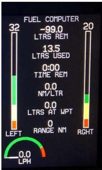
This page displays fuel tank levels, fuel flow, fuel pressure, fuel remaining, fuel used, and time remaining.
