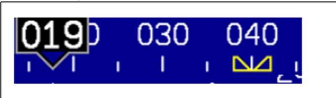
When the AP is not engaged for a given axis, the respective BUG is hollow.
