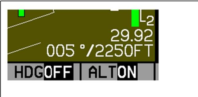
Whenever either the heading or altitude Bug is toggled ON, its current value is displayed in the lower right corner of the EFIS page.
