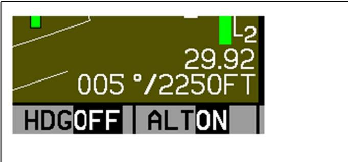
Whenever either the heading or altitude Bug is toggled ON, its current value is displayed in the lower right corner of the EFIS page.
