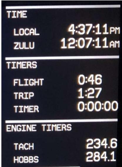
The Times Page is divided into three sections: TIME, TIMERS, and ENGINE TIMERS.
